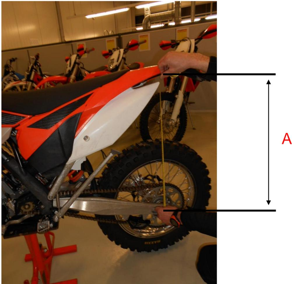
Determining the static sag of the shock absorber:
